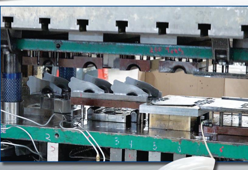
With production stamping presses ranging from 20 ton to 400 ton, K-TEK has the capability to handle Short Run, Progressive Die Stamping, and your full tooling needs.
